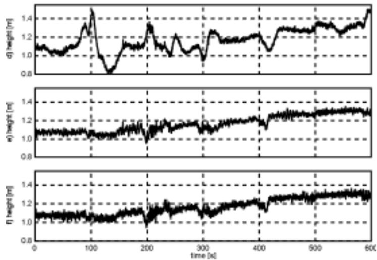
In fig. 2 the heave as obtained from different methods has been subtracted from the RTK height. The graphs should therefore show the mean vertical position after heave compensation. The difference between the heave-corrected RTK-height and the smoothed result shown in graph c) of fig. 1 can be used to calculate a comparable standard deviation for the different methods. The standard deviation of the initial RTK-height in plot a) of fig. 1 is derived as 4.1 cm.
