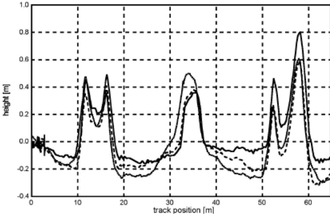
Fig. 4 shows results for the passage of the cart over a series of humps on a straight section of the course. Speed was approximately 1.5 m/s. Height as determined by DGPS with the nearby stationary reference receiver is indicated by the solid curve. The quality of this solution was checked to be better than 1.5 cm. Both of the independent methods of heave determination have been applied to this case and will now be discussed.
